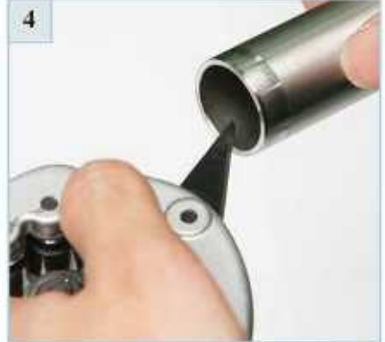
Lightly de - burr inside and outside edge. Bevel up to 0.3mm X 45° (0.012° X 45°) permissible.
