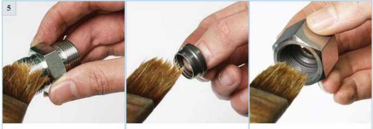
Lubricate thread and cone of fitting body, also cutting ring and thread of nut.
